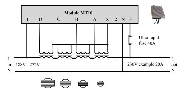
Use an ultra fast fuse. A standard fuse or no fuse may destroy a module. Check connections before turning on. Use quality connector terminals only. If switches, use quality spring-loaded ones only.
