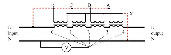
Apply 230V to the input. If the output is 42V lower, remove dotted wires and go to the next page.
