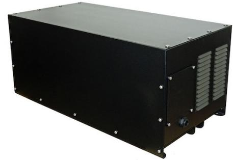
A MultiPhase converter converts single-phase into three-phase power much like a Booster converter. The MultiPhase has an additional nine stage power electronic system which balances the output voltages precisely over the whole range of different loads.
