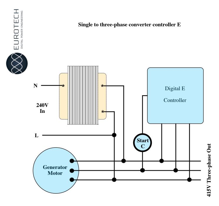
The input voltage is stepped up to 415V (not required in US versions).
