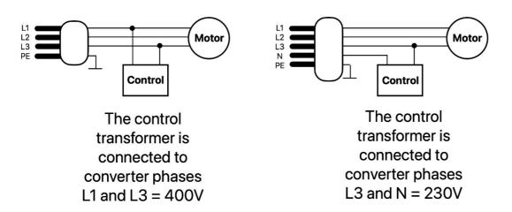
Rotate wires L1 L2 L3 in the plug of a machine until this is true
