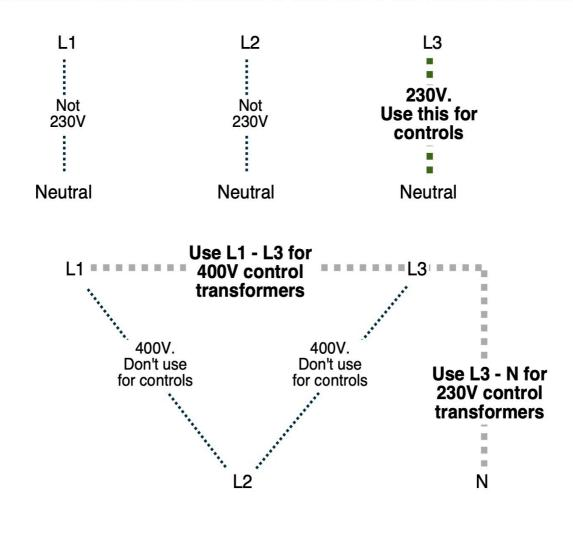
If machine has a four pin plug
