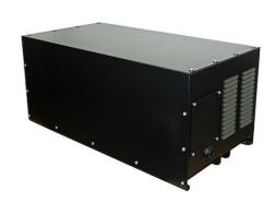
A MultiPhase converts single-phase into 400V three-phase voltages. An ideal choice for machines with three-phase motors connected to inverters, such as in CNC machines. The digital power electronics recognise starting motors and generate the currents to accelerate all motors as fast as if they were connected to the three-phase mains. The three-phase voltage symmetry is electronically maintained at all loads. Leading converter manufacturers world wide use our electronics in their products.
